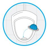
b) Place a blueFox1 bio-capsule over the drain outlet in each bowl with the semi-circle pointing up.
