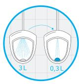
c) Regulate the water volume for flushing to 0.3 litres. This achieves a 90% water saving with every flush.
